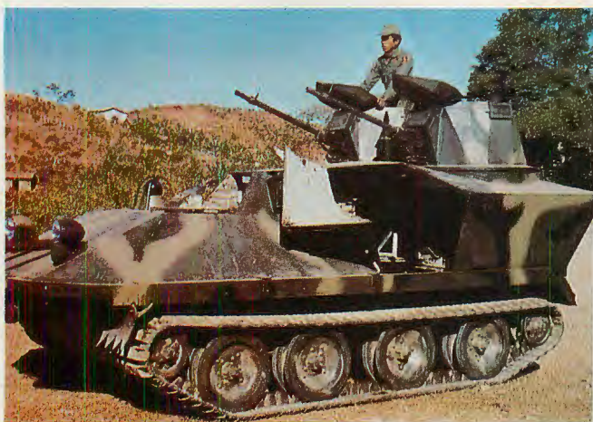
ABOVE AND RIGHT: M114 track with Salvadoran face-lift sports M2 .50-cal. Browning aircraft machine guns.
